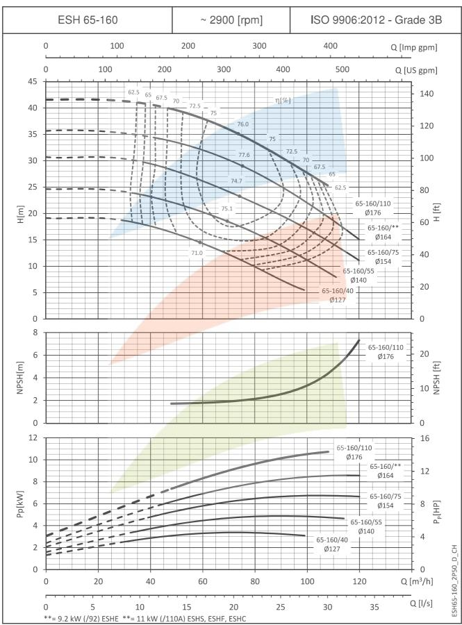
The NPSH values are laboratory values; for practical use we suggest increasing these values by 0,5 m. These performances are valid for liquids with density  $\rho=1,0~\text{Kg/dm}^3$  and kinematic viscosity  $\nu=1~\text{mm}^2/\text{sec}$
